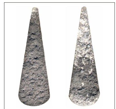
Figure 1. Chill removal with 0.1% Superseed Extra inoculant (left) as ladle addition compared to 0.1% F.G.FeSi (right) in 0.04% sulphur base iron
